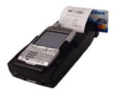
The PP-55 makes your PDA/Smartphone a more powerful tool. Simply slide your handheld into the PP-55's custom cradle and create a powerful, portable enterprise solution. The standard PP-55 allows you to print information from your handheld. The PP-55MS integrates a three track magnetic stripe reader. The PP-55MS-BC integrates a Symbol® CCD barcode scan engine with the printer and mag stripe reader.
