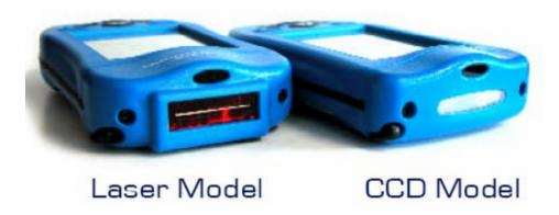
Both laser and CCD based barcode reader modules are available for the Aceeca Meazura RDAs (ruggedized digital assistants).
